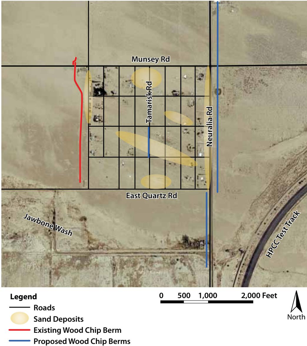
**Figure 15:** Diagram of Rancho Seco showing front line wood chip berm to the west, the remaining sand deposits within Rancho Seco, three proposed additional berms and the northwest edge of the 7-mile HPCC test track east of Neuralia Rd.
