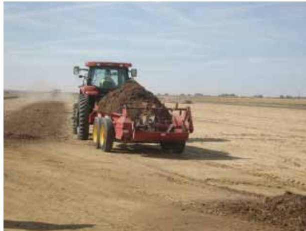
Figure 9: A fertilizer spreader can be used to cover bare soil with a layer of wood chips.
